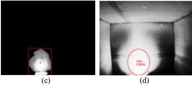
Fig. 4. Results of the object detection by image processing and probabilistic classification by Bayesian classifier. (a) original visual image, (b) original thermal image, (c) background subtraction and object detection result, and (d) classification result in a room where a fire is present.
