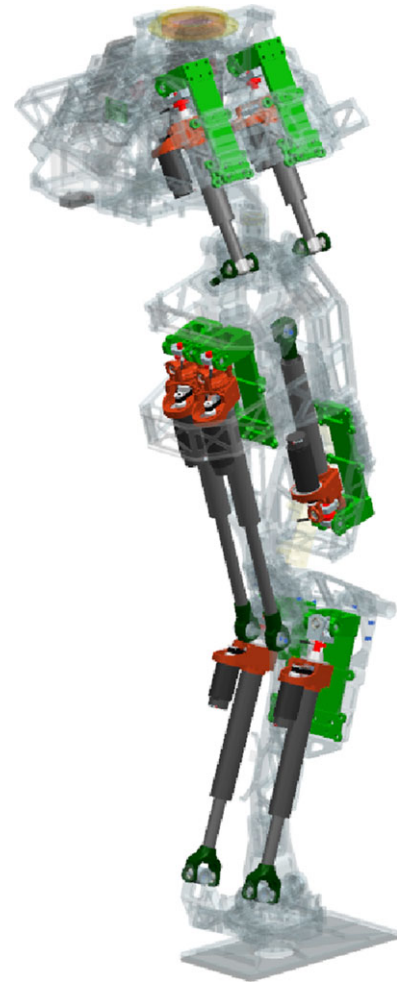
Figure 3. Rear view of ESCHER's right leg showing the placement of the linear SEAs.
